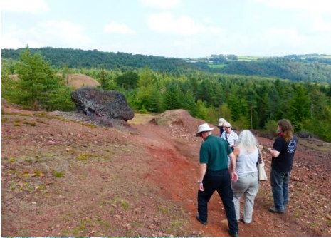
Part of the waste dumps - the black lump is called 'winkle' and came from the arsenic calciner, while the red finer material came from the ore itself.
