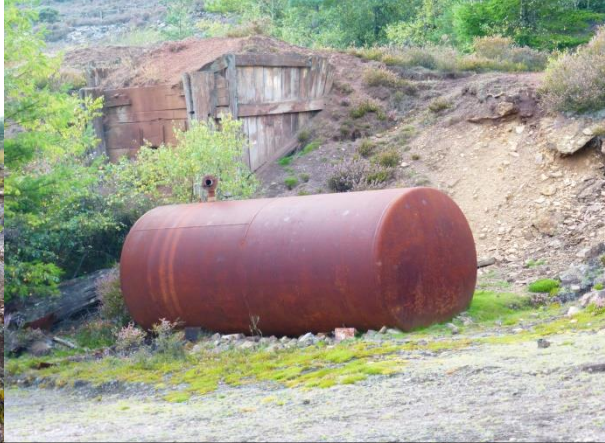
The water tank for the jigger from the 1970s and the wooden scaffold to support the jigger behind. The jigger acted as a gravity separation sieve, separating material of the same size
