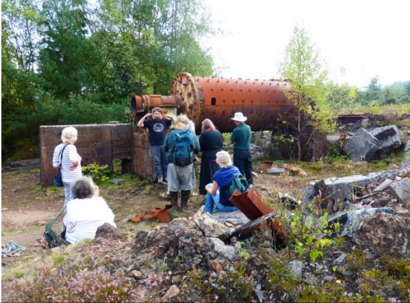
Ballmill crusher from the 1970s – this was filled with ball bearings to crush the waste more finely to recover the mineral. Some of the ball bearings were lying on the ground
