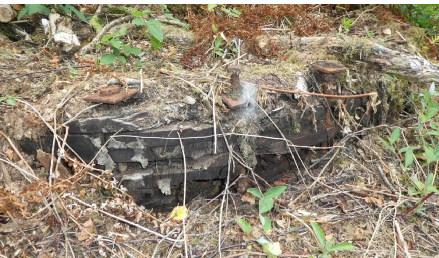
below: The outside of the wheel rim made up of small sections of wood held together with iron fixings, 14 July 2018
