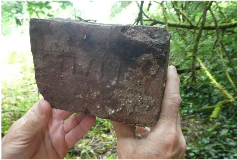
A broken brick from Bealswood Brickworks inscribed (WE)STLAKE. These bricks were red with no frog, July 2019.
